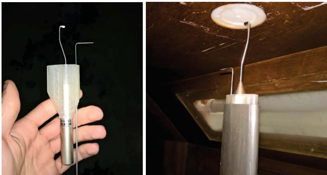
Figure A.10: Rapid prototyped Cobra probe holder (left) fitted to streamline tube in tunnel (right).
