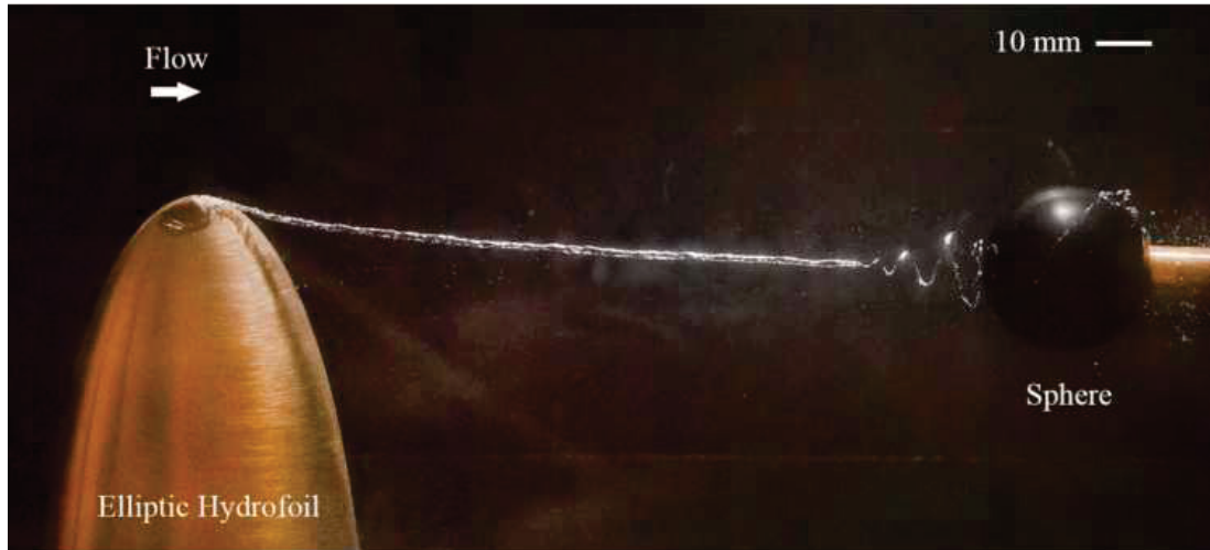
Figure 2.27: Interaction of elliptical wingtip vortex with sphere in the wake, reproduced with permission from Pasche et. al. [32]
