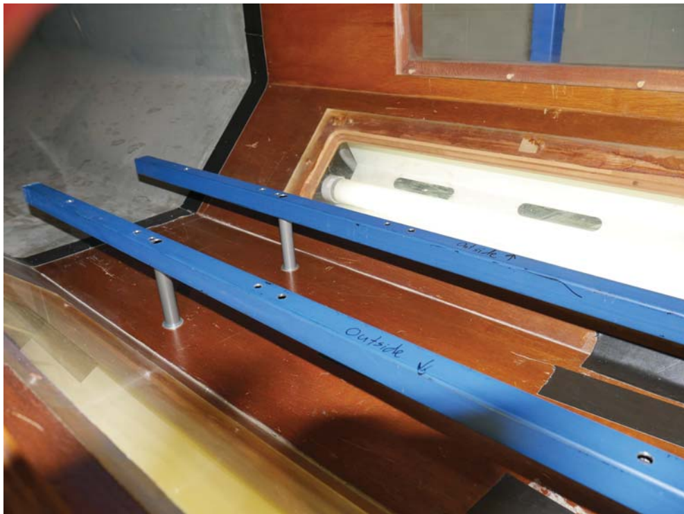
Figure A.1: Detail of mounting rail, with plate mounting holes shown.
