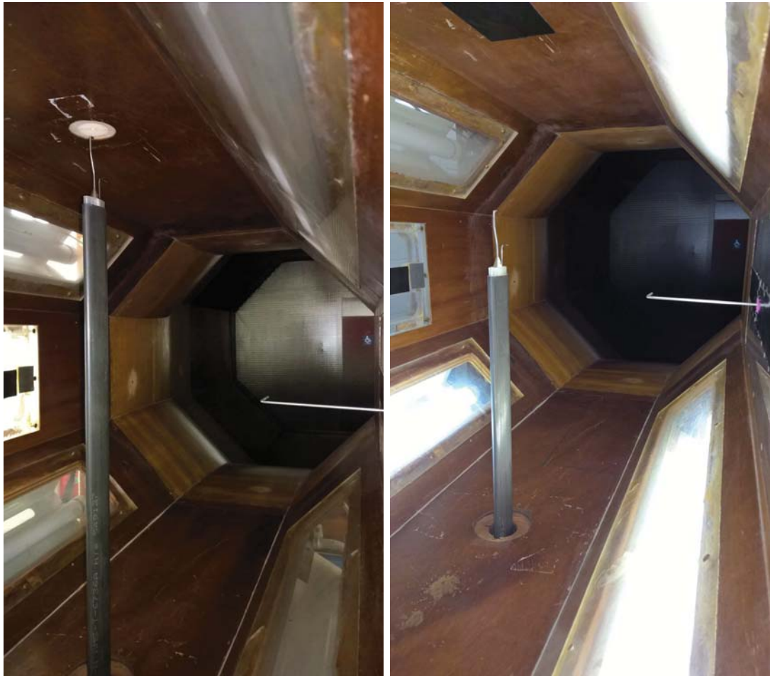
Figure A.11: Pitot tube arrangement for characterisation of tunnel flow, with traverse up (left) and midway through tunnel (right).
